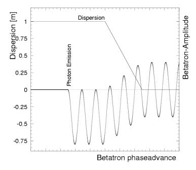
For an ideal, flat accelerator the vertical dispersion is zero, i.e. there is an extremely small vertical emittance. In an accelerator with errors, coupling and spurious vertical dispersion increase the vertical emittance.
