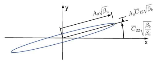
Again driving terms scale like the sqrt of the product of the beta functions at the location of the skew errors.
