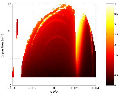
Tracking results are in good agreement with measured effects, i.e. case with dispersion wave has less yellow and orange areas than the one with excited coupling resonance, indicating less sensitivity to reduced vertical aperture
