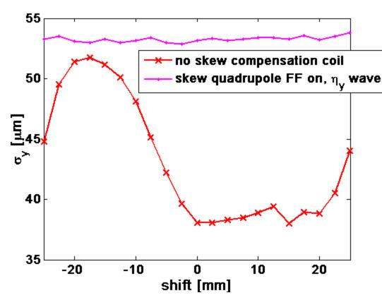
For reference: Whenever an undulator moves, about 120-150 magnets are changed to compensate for the effect (slow+fast feed-forward, slow+fast feedback)
